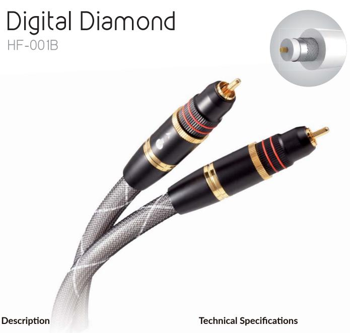
The coaxial constructed RCA HiFi digital signal cable HF-001B has a multi-strand internal conductor structure having a 0.6333 mm<sup>2</sup> cross-section, made from high-quality copper using OCC® (Ohno Continuous Casting) technology and having a material purity of 99.9999%. The shielding is constructed using aluminum foil and tinned copper braiding. The contact surfaces of the RCA plugs (m/m) are 24k gold plated for absolute corrosion resistance and loss-free signal transmission.
